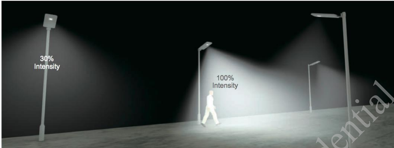
Solar lights works at dim mode when humans are not around. Integrated Passive Infrared. Sensor to increase light output when motion is detected.
